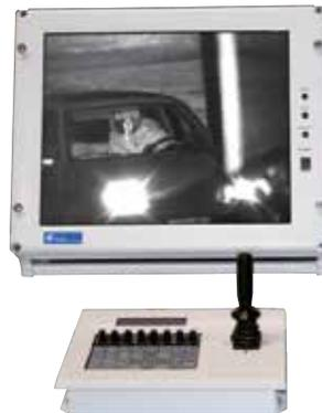
The ALI operates under any illuminations condition ranging from complete darkness to bright sunlight, even in presence of fog, rain or smoke.
