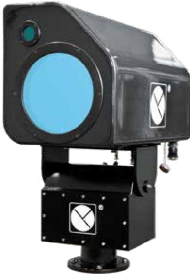
The Active Laser Imaging (ALI) system is an active system utilizing an eye-safe infrared laser beam (1550 nm wavelength) to illuminate a target and a Focal Plane Array (FPA) to collect the backscattered radiation.
