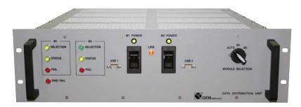
The IU80-25 unit provides sensor data integration and distribution over a network. It is equipped with a number of ports, which can be connected with a wide range of marine navigation sensors compliant with IMO interface regulation IEC-61162. The embedded CPU decodes all messages coming from and going to ship sensors, encapsulates them into Ethernet packets and deliver over the IBS LAN.
