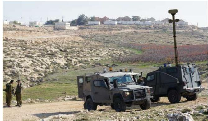
DEFENDER structure allows radar and Night/Day camera surveillance over 360° with pan and tilt capability: the radar and cameras can be mounted on the same side of the mechanism, as the radar equipment is free from any interference. Additionally, the cameras can also operate independently from the radar.
