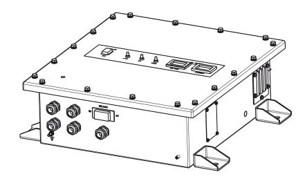
The IU80-30 unit provides 27 VDC output, internally battery backed for uninterrupted power supply. DC voltage is generated from AC voltage input. Battery size guarantees more than 1 hour of power supply output in case of input mains loss. It also provides continuous monitor of output voltage and current.
