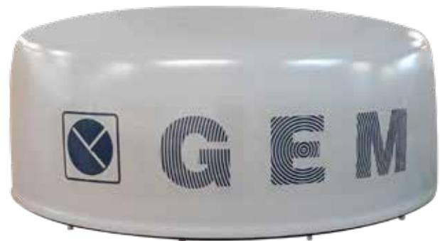
**Sea Eagle-50/RD** belongs to a new generation of solid state radar specially designed for naval applications. The radar sensor is a pulse compressed X-band transceiver. Lower power selections together with special waveform combination allow the radar to see without being seen. Moreover a sophisticated anti clutter rejection achieved by using video and Doppler processing is an embedded feature for the detection of small targets.
