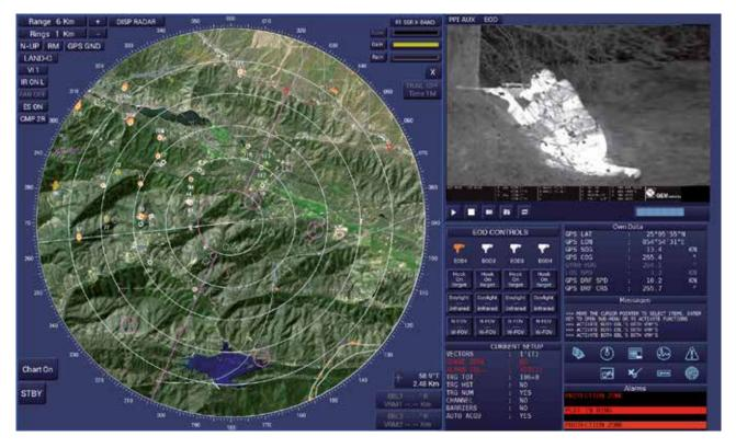
GEM DEFENDER control and display software can integrates multiple sensors, such as radars and camera, into a single, easy to use display package. The management application software allows the operator to get a real-time situational awareness by early detection of possible threats and will provide "actionable data" to launch prompt response missions and counter measures. The system makes the tracks "fusion" of geo-referenced radar tracks from multiple radar heads into one user-friendly display.
