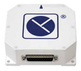
MRS-011 is an attitude measurement system based on high quality MEMS sensors, integrating GEM proprietary algorithms based on Kalman Filters for platform attitude over time, the calculation of heading and the routing of navigation data coming from the GPS/DVL/USBL.
