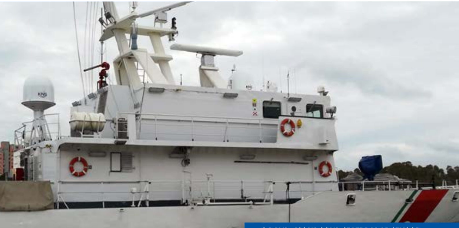
S-BAND 400 W SOLID STATE RADAR SENSOR
